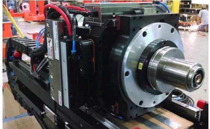
LASER TRACKER GUIDED X-Y MICROPOSITIONING DRILL SPINDLE
