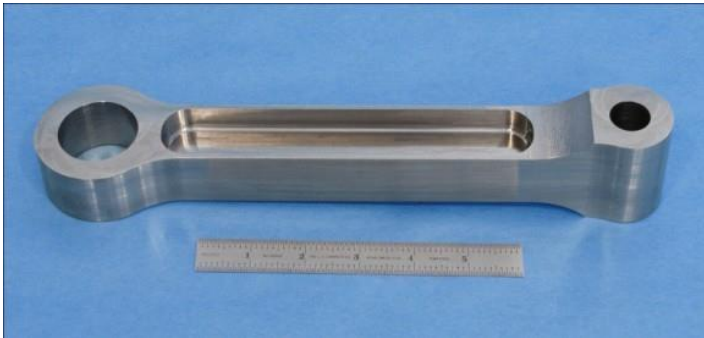
Representative F-35 Part Machined 2X Faster with Cryogenic Machining
