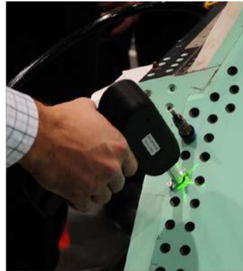
MANUAL HOOK GAUGE – WIRELESS GRIP GUN AND F-35 FASTENER LOCATION
