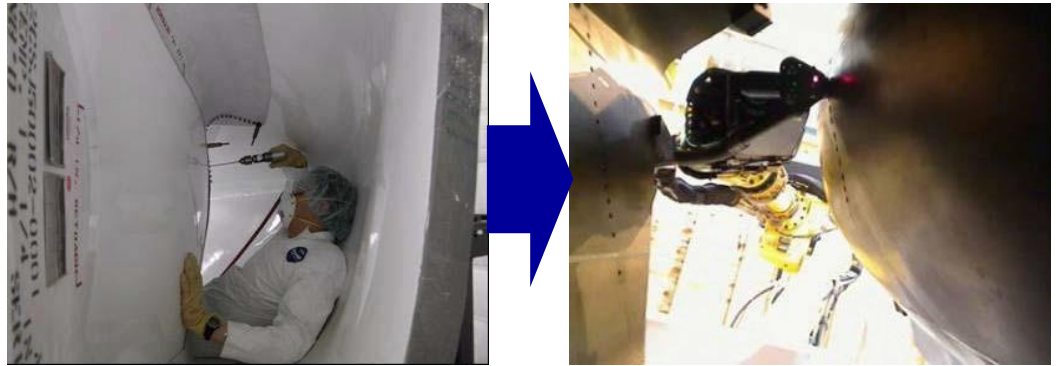
F-35 INLET DUCT DRILLING – MANUAL (LEFT) AND AUTOMATED (RIGHT)
