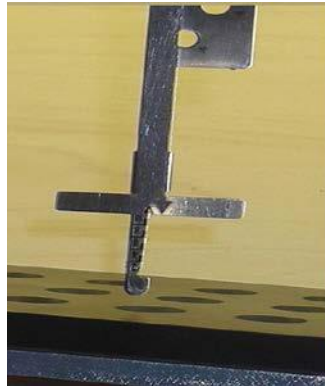
MANUAL HOOK GAUGE – WIRELESS GRIP GUN AND F-35 FASTENER LOCATION
